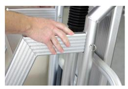
Align the mounting holes of the ladder over the ladder mounting holes and secure the ladder to the plates using eye bolts.
