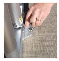
**Step 12.** Install your assembled diving board using the eye bolts to secure the frame and ladder to the mount plates.
